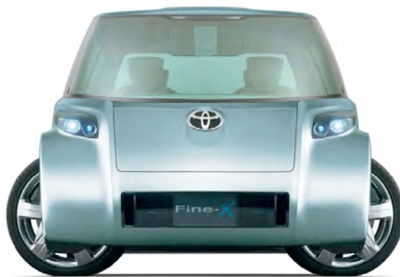
Figure 7: Toyota Fine-X concept car having 4 in-wheel electric hub motors
